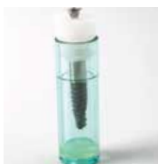
The methacrylate vial with Polyethylene (PE) top is carefully washed and dried.
